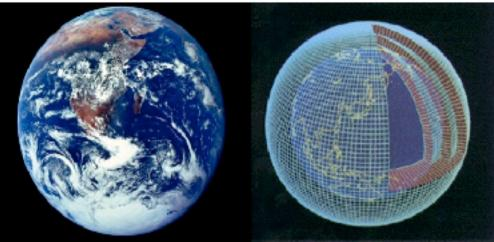
Dynamics: solve the 3-D equations of motion on rotating sphere Physics: parameterize sub-grid phenomena on vertical profiles, → turbulence, hydrological processes,
